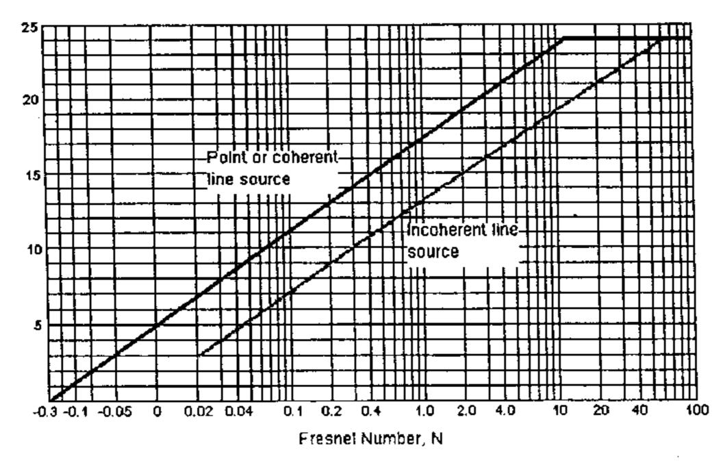
The total attenuation of the barrier is given by the following equation (Beranek 1971):
