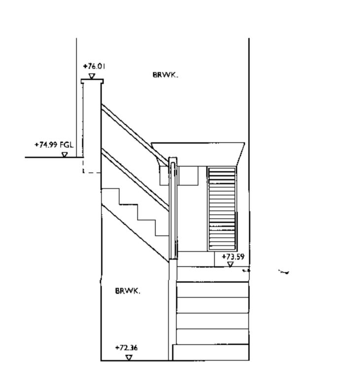
SECTION DETAIL D-D THRU' FLAT 9 ENTRANCE AS EXISTING. SCALE 1:50
