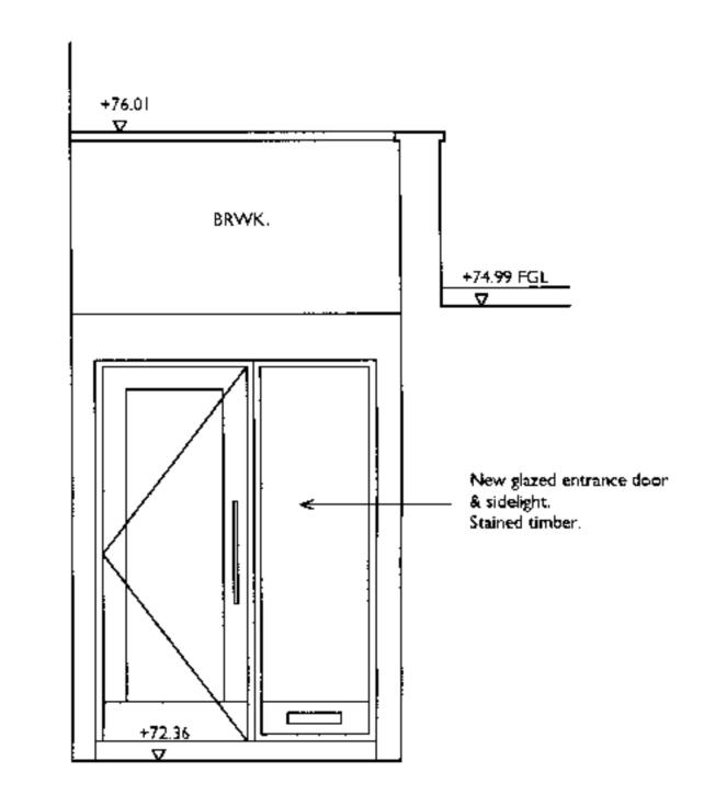
SECTION DETAIL C-C THRU' FLAT 9 ENTRANCE AS PROPOSED. SCALE 1:50
