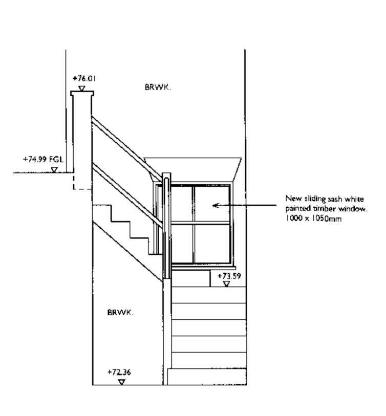
SECTION DETAIL D-D THRU' FLAT 9 ENTRANCE AS PROPOSED. SCALE 1:50
