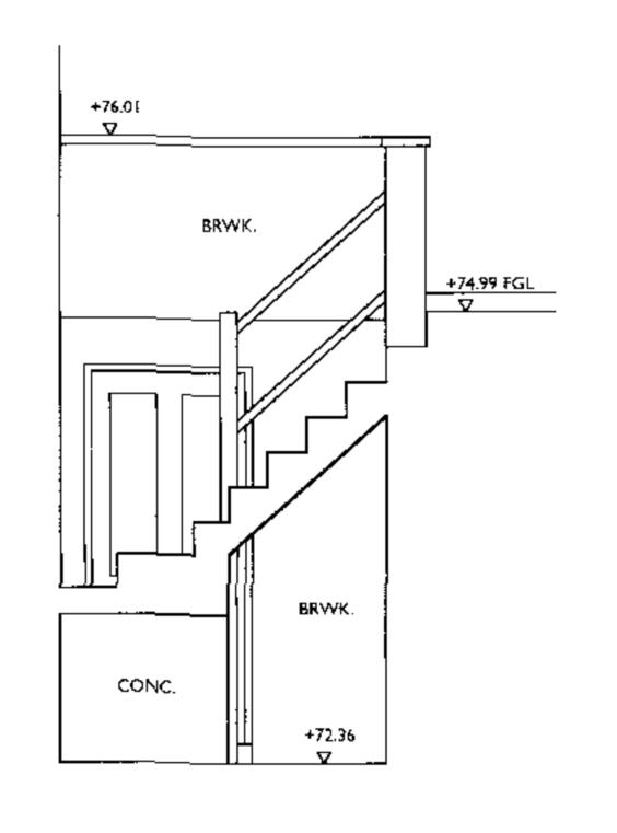
SECTION DETAIL B-B THRU' FLAT 9 ENTRANCE AS EXISTING. SCALE 1:50
