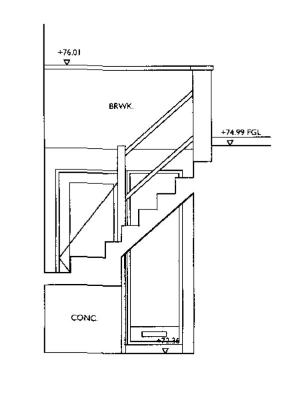
SECTION DETAIL B-B THRU' FLAT 9 ENTRANCE AS PROPOSED. SCALE 1:50
