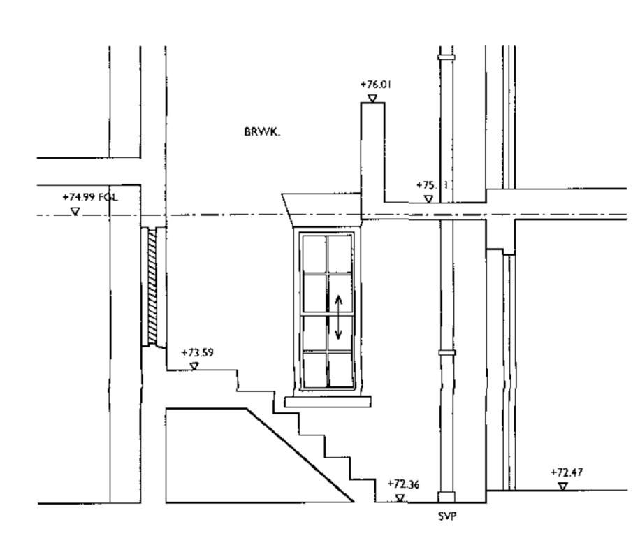
SECTION DETAIL A-A THRU' FLAT 9 ENTRANCE AS EXISTING. SCALE 1:50
