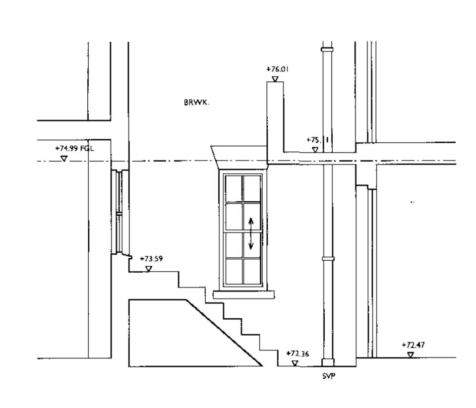
SECTION DETAIL A-A THRU' FLAT 9 ENTRANCE AS PROPOSED.
