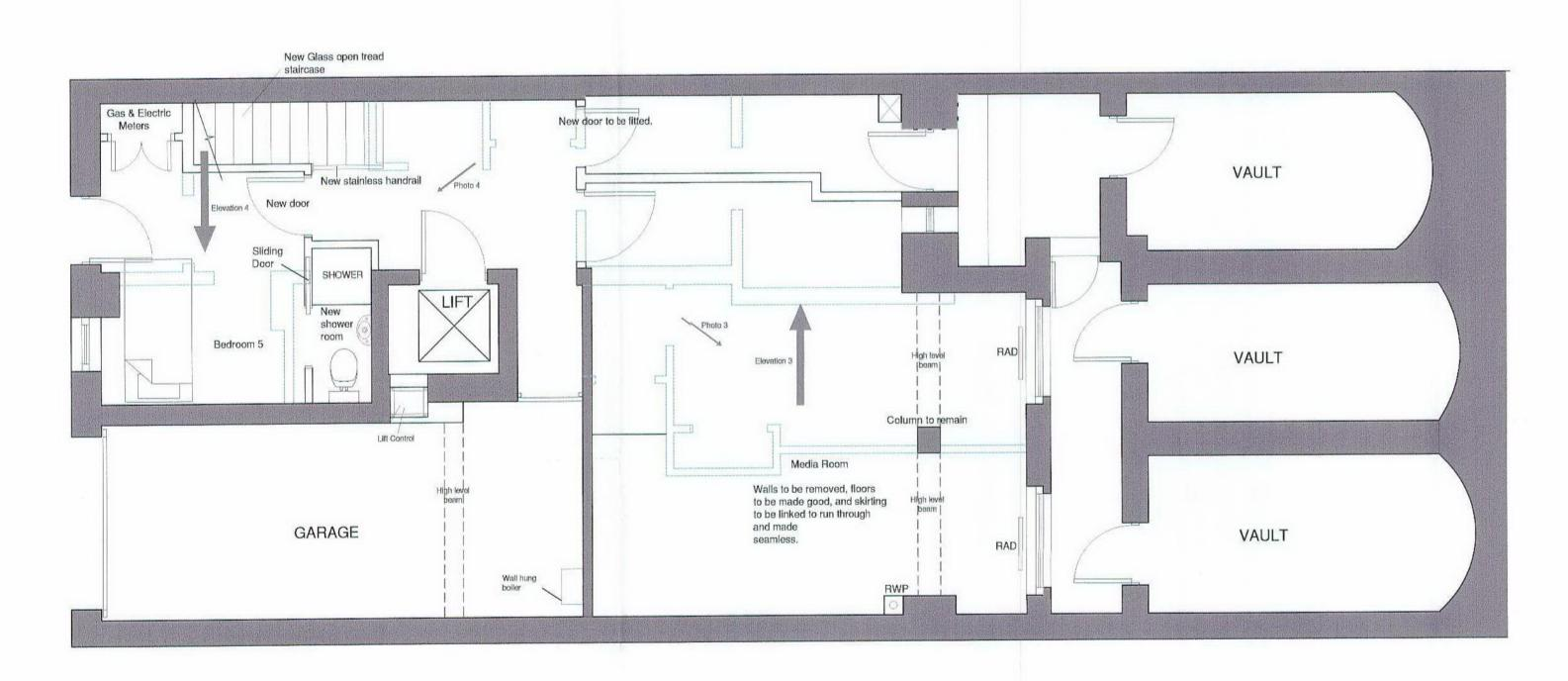
Where walls were removed form new media room, floors walls are to be made good, skirting to be linked to run and made seamless. New stud wall to be constructed to form new media room which will be finished to match existing wall finish and skirting. Walls are to be finished to r the existing basement walls currently have a paint finish Proposed Elevation
