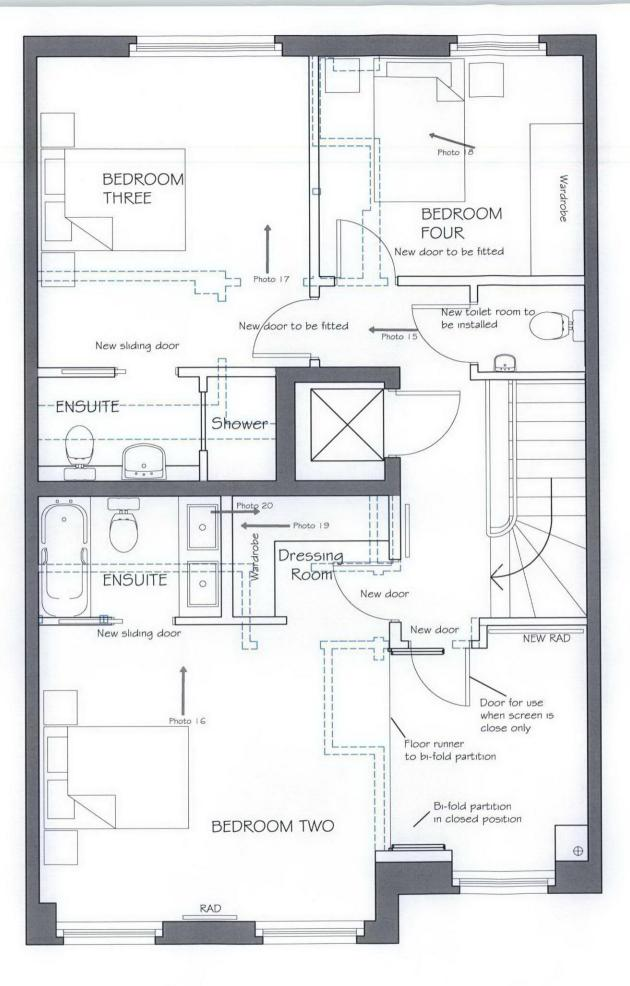
Walls and fitted cupboards to be removed, floor to be made good with skirting linked and made seamless. New stud walls with plaster finish installed.
