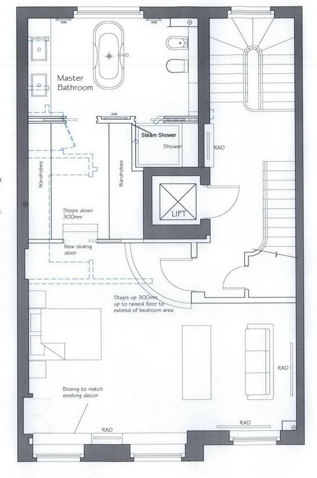
Existing walls and fitted wardrobes to be removed floors to be made good, skirting to be linked and made seamless with new stud walls and fitted wardrobes to be installed.
