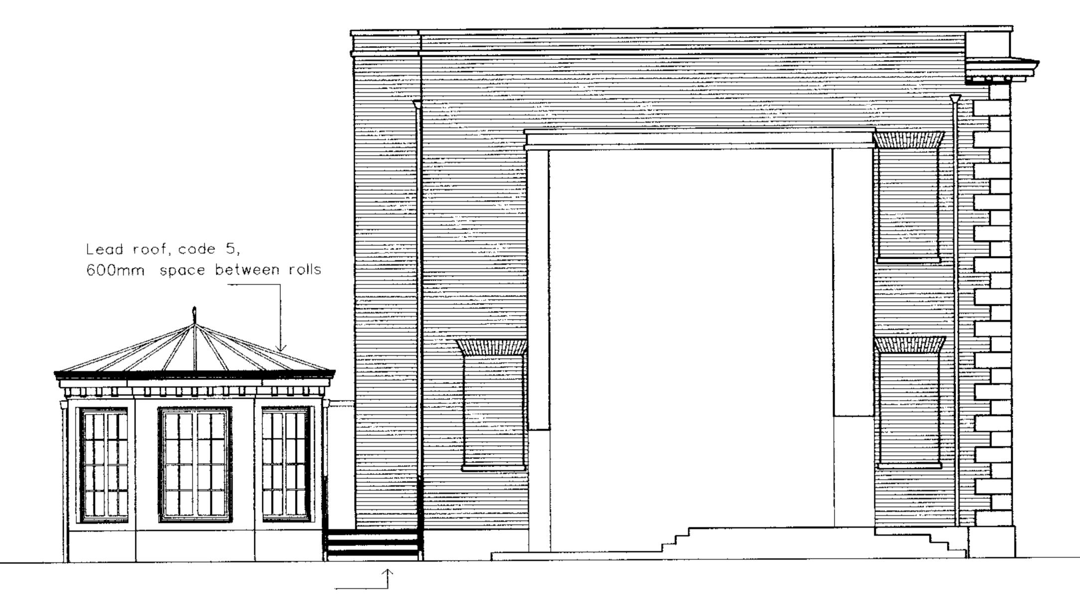
External steps to be full deck width & to have 100mm open risers for ventilation of Condenser Unit located below deck
