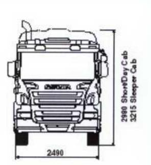
AB (centreline of front axle to back of cab) Short - 300 Day - 590 Sleeper - 960 \*Reduces to 250mm with sleeper cab
