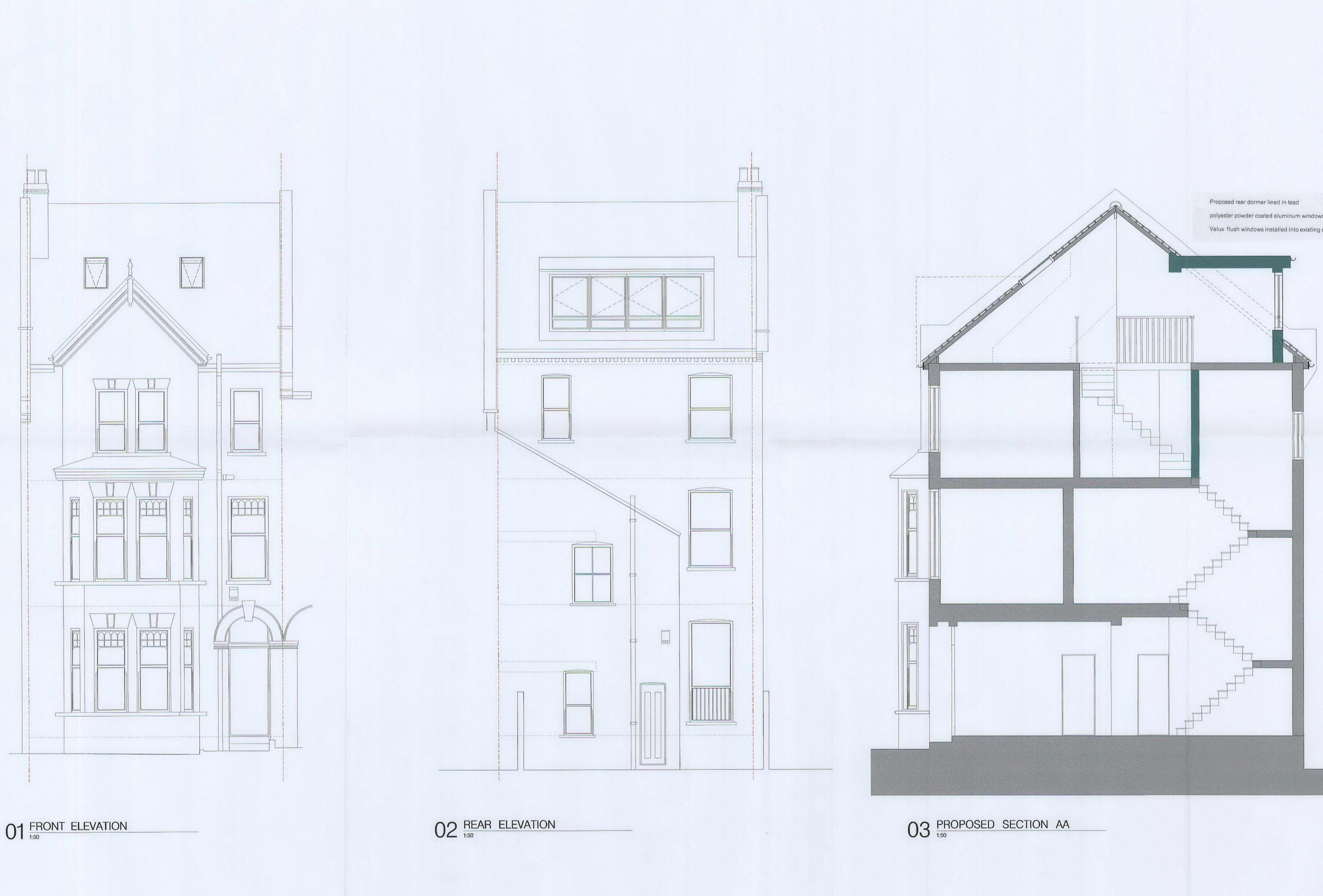
polyester powder coated aluminum windows Slate roof to rear retained wherever possible Velux flush windows installed into existing slate tiled roof to the front of property KEY PLAN JAMES BURGE 19 HEATH HURST ROAD LONDON NW3 2RX Mario Pilla Architects STATUS 0019 -PA-020
