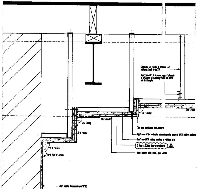
DETAIL 5 - Section - Type C2 stepped MF ceiling along Section MM
