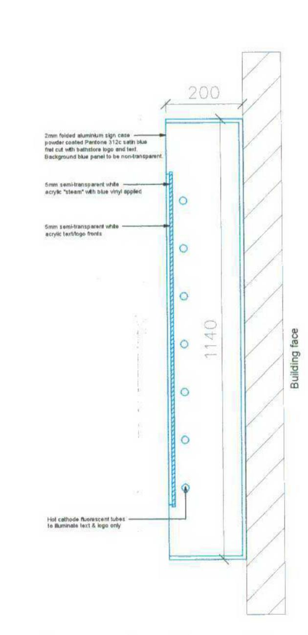
Section through internally lit fascia sign - scale 1:10 Box sign with fret cut text & logo
