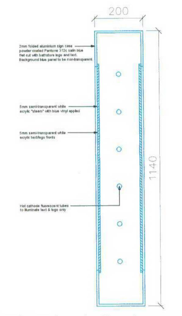
Section through projecting sign - scale 1:10 Box sign with fret cut text & logo
