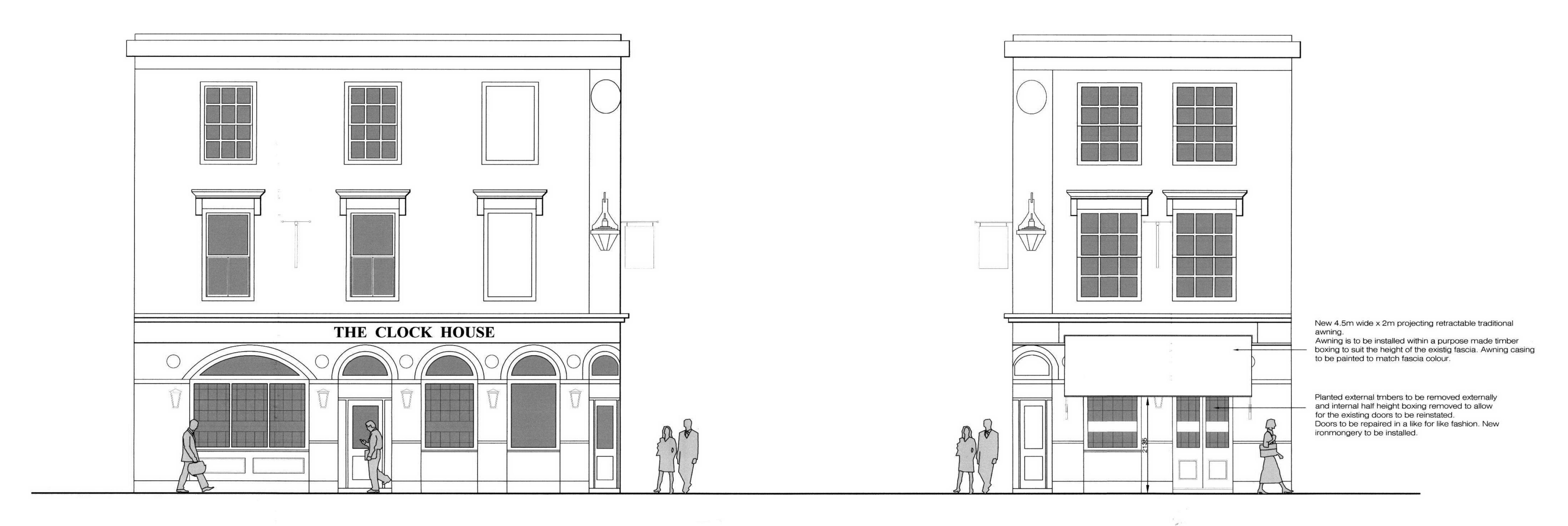
PROPOSED ELEVATION to HATTON WALL scale 1:50
