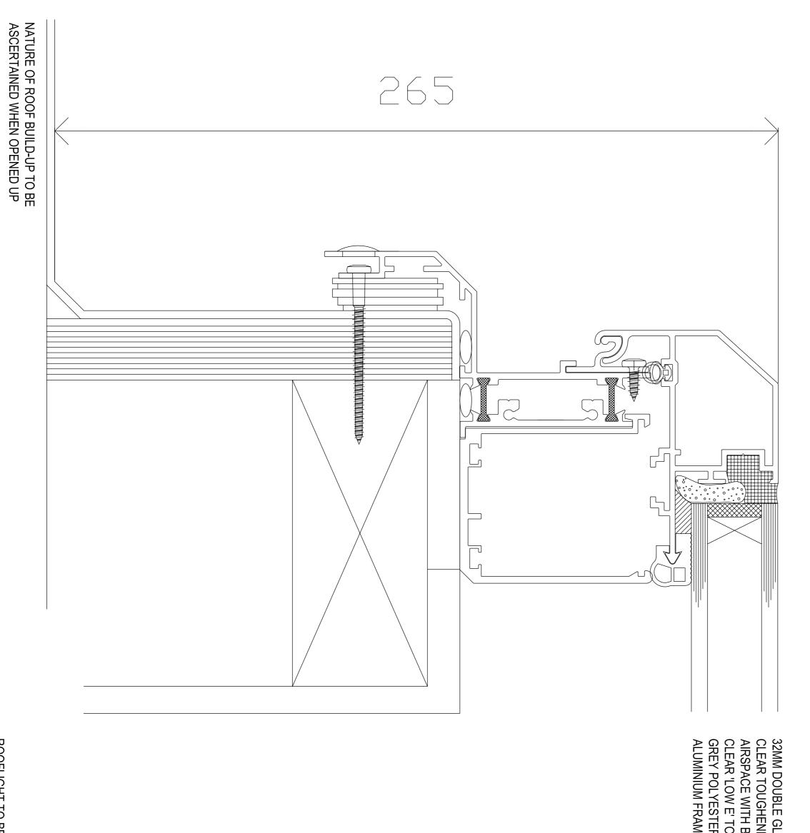
ROOFLIGHT TO BE CONSTRUCTED AS A SQUARE WITH THE SMALLEST DIMENSIONS WHICH WILL FIT AROUND THE EXISTING CIRCULAR OPENING
