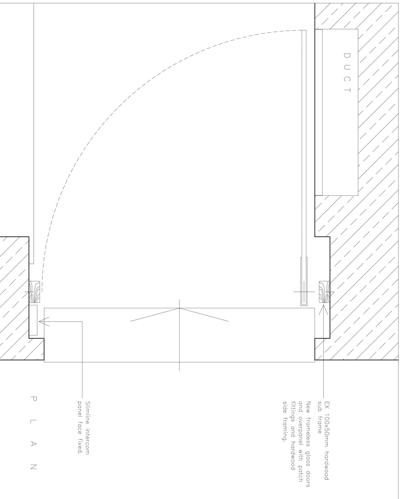
Manufacturer's detail of floor hinge patch plate, and floor closer. Carefully form opening in floor, and fix as directed by mfr. Timber frame plugged and screwed to wall, at approx 300mm centres.
