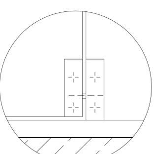
Stainless steel top patch hinge detail
