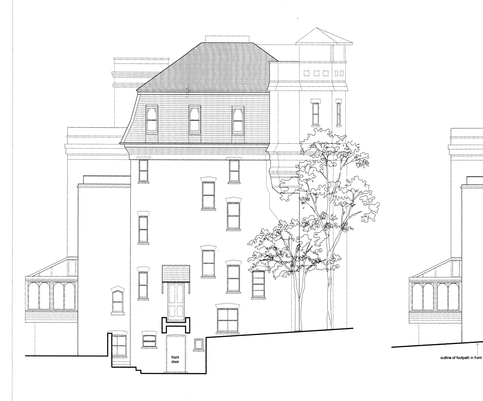
east sectional elevation as existing (true elevation into front area)
