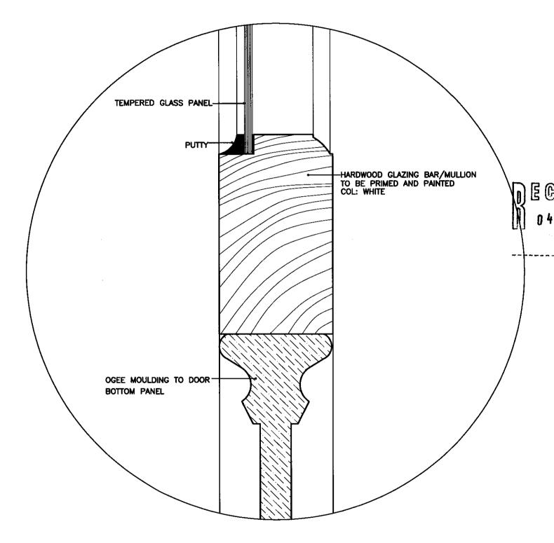
PROPOSED NEW EXTERNAL DOORS DOOR TYPE D; GLAZING BAR AND BOTTOM PANEL DETAIL
