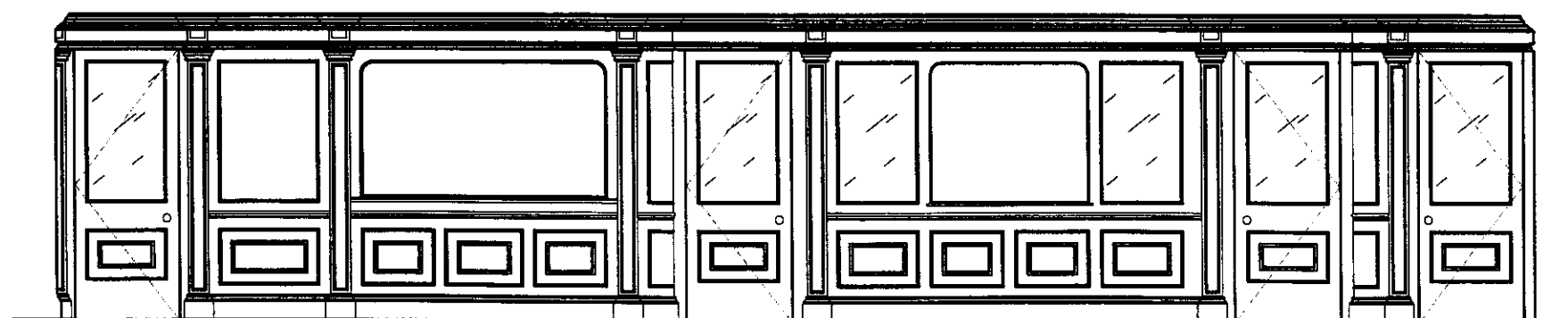
14 0423 ELEVATION 14 TIMBER WALL SCREENS TO BE REMOVED
