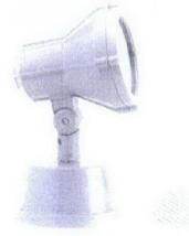
C and D - ALC Veola Compact Architectural Spotlight 6° with 35W/70W warm white metal halide for column lighitng, with spread lens for facade life expectation of 100,000 hr. and ledge line lighting. With filter colour as an option.
