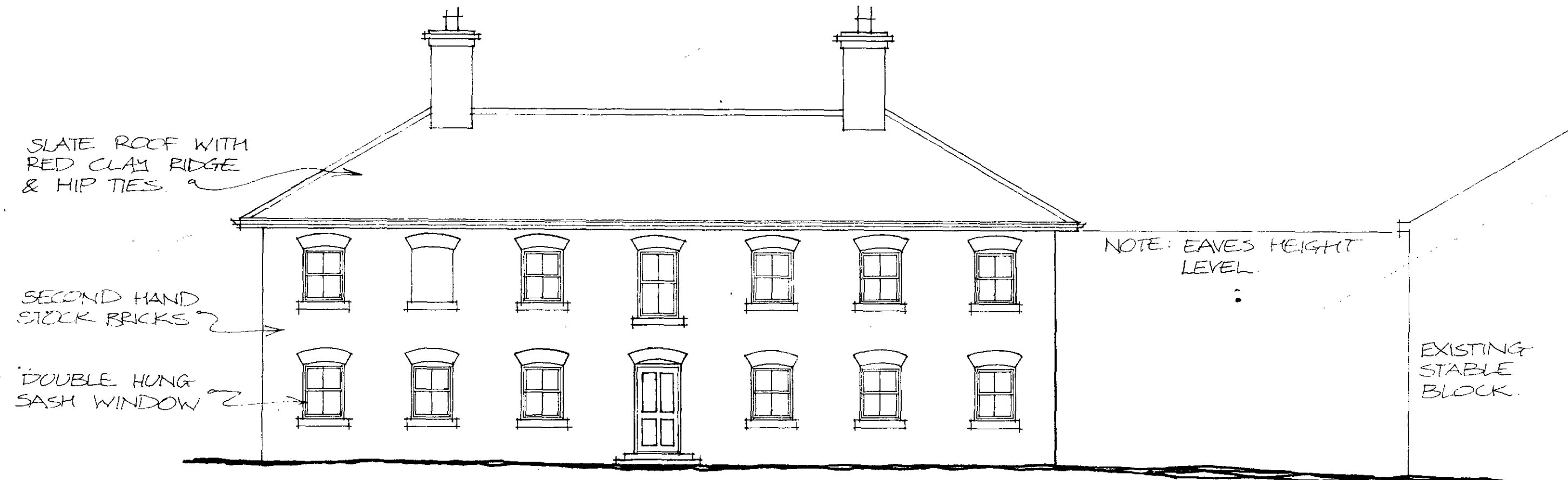
5 NORTH WEST ELEVATION 1:100
