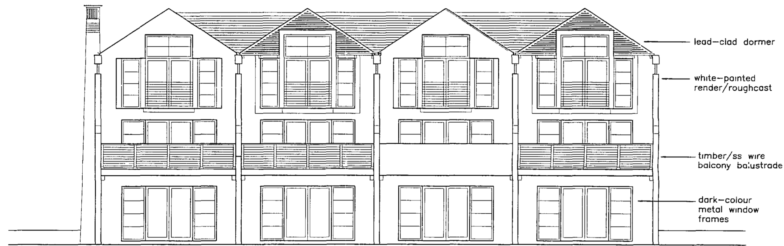
UNIT 1 UNIT 2 UNIT 3 UNIT 4 SOUTH-EAST ELEVATION
