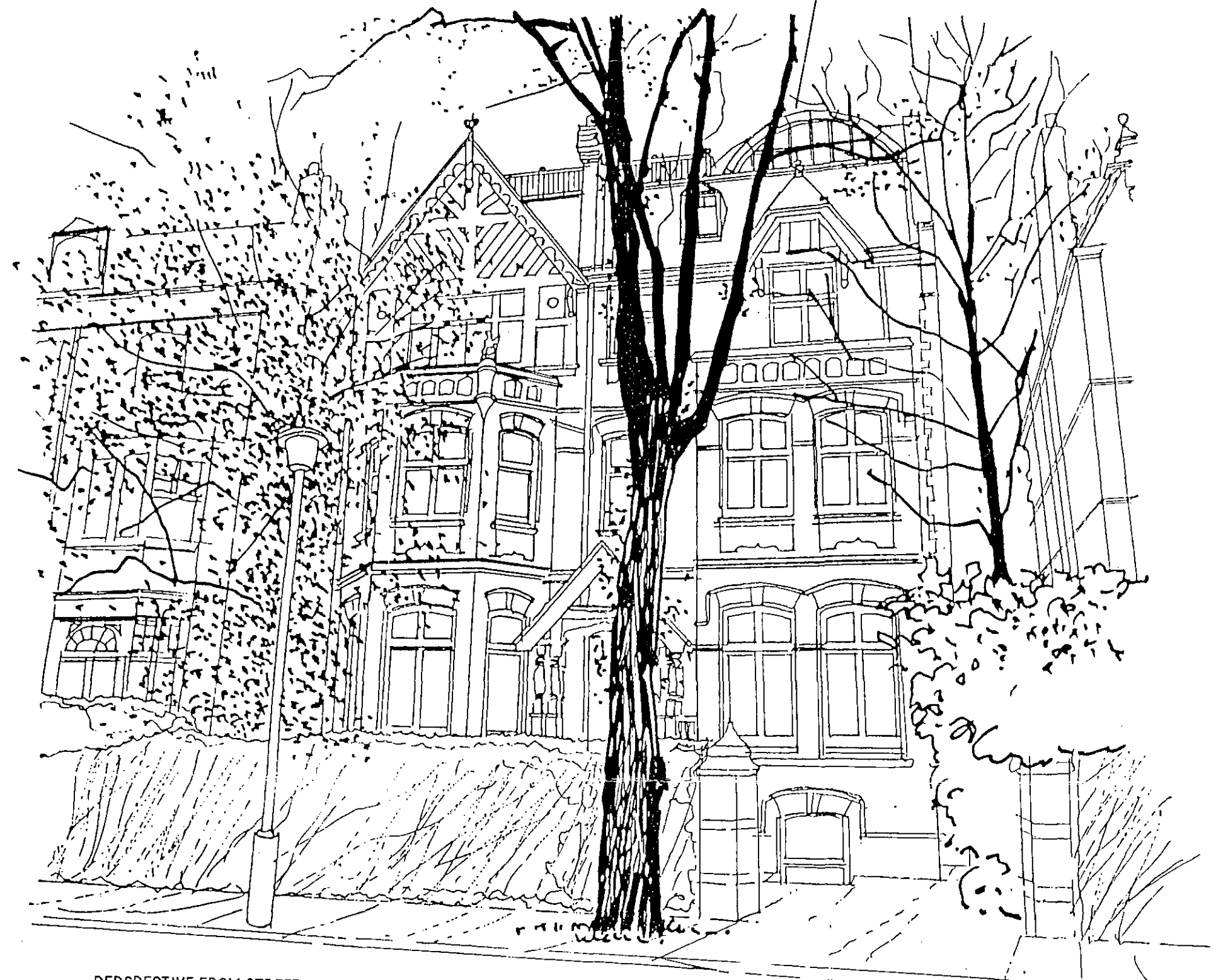
PERSPECTIVE FROM STREET LEVEL - WITH ROOF EXTENSION. NB - The barrel vault reduces the impact of the design from street level.
