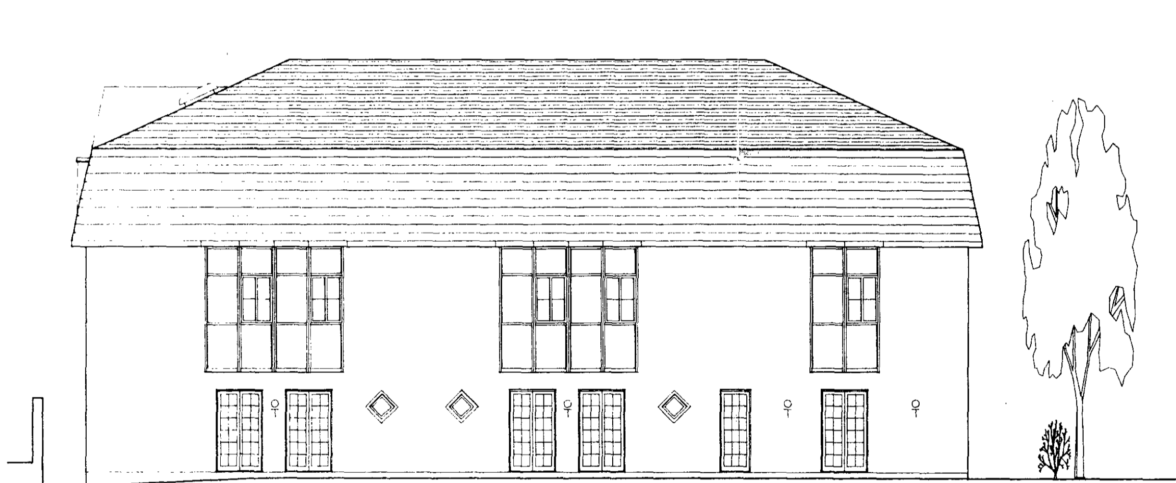
East Elevation (West is same but handed)
