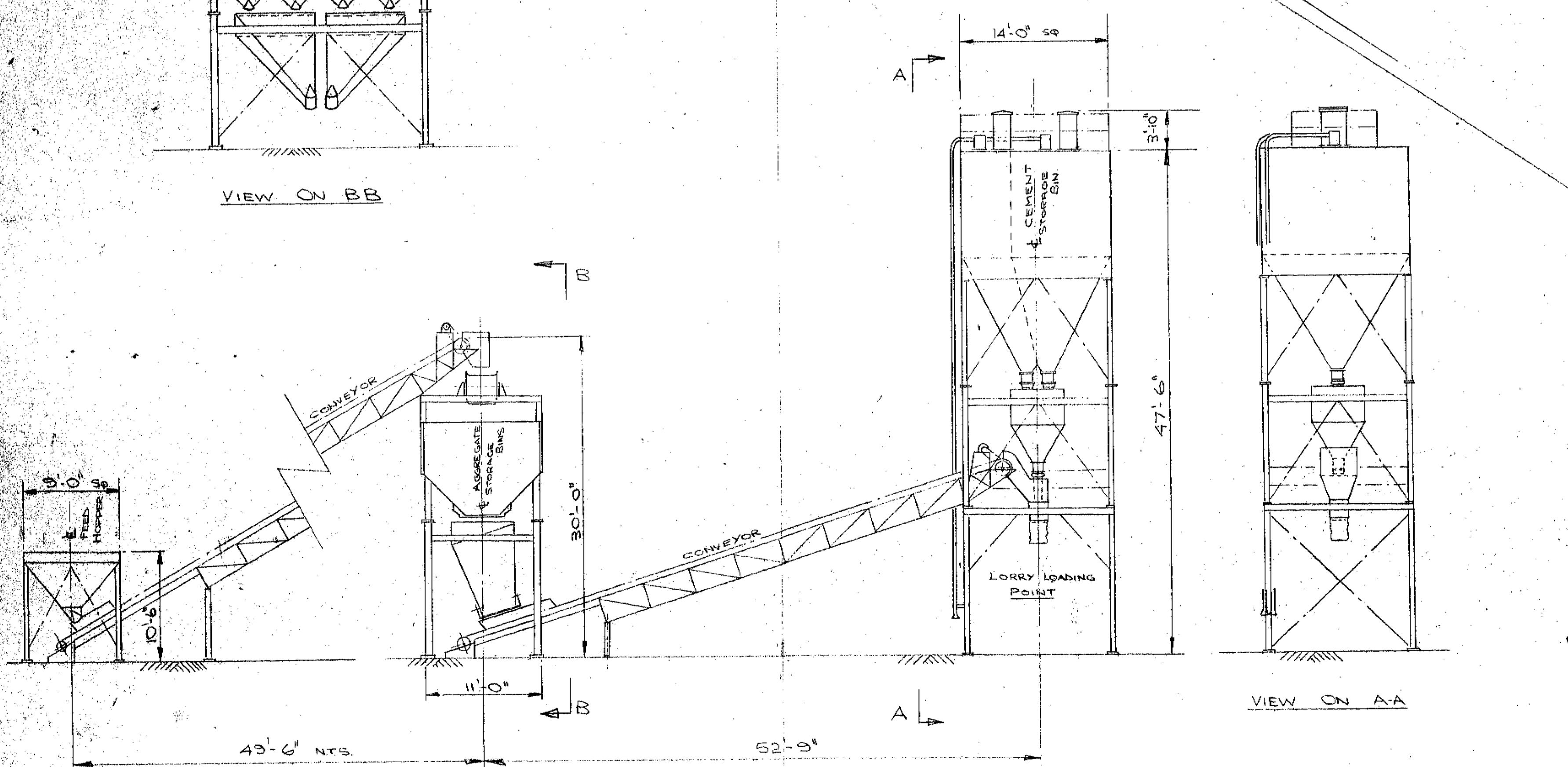
ELEVATIONS ON BATCHING PLANT
