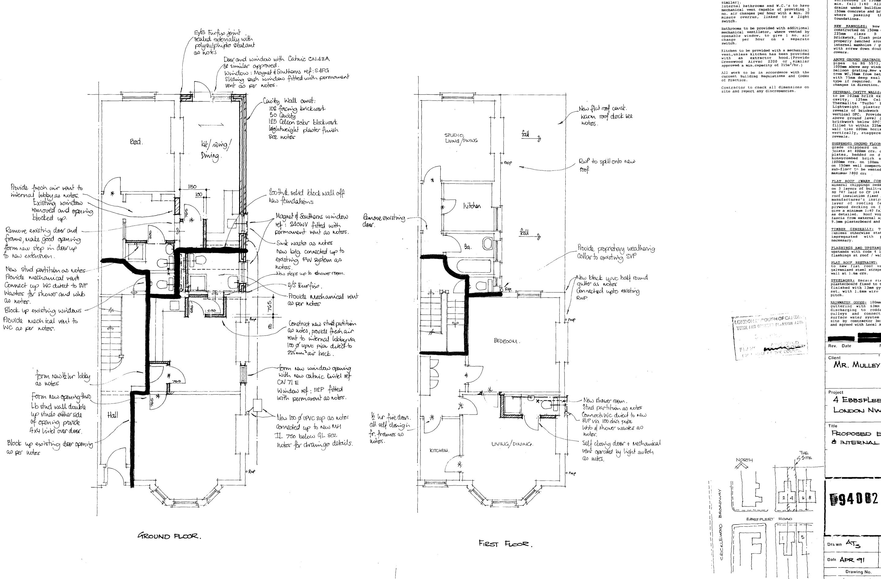
TIMBER PARTITIONS Studs to be 75mm x 50mm @ 400mm crs. with 75mm x 50mm head & sole plates.(2.4m high max.)
