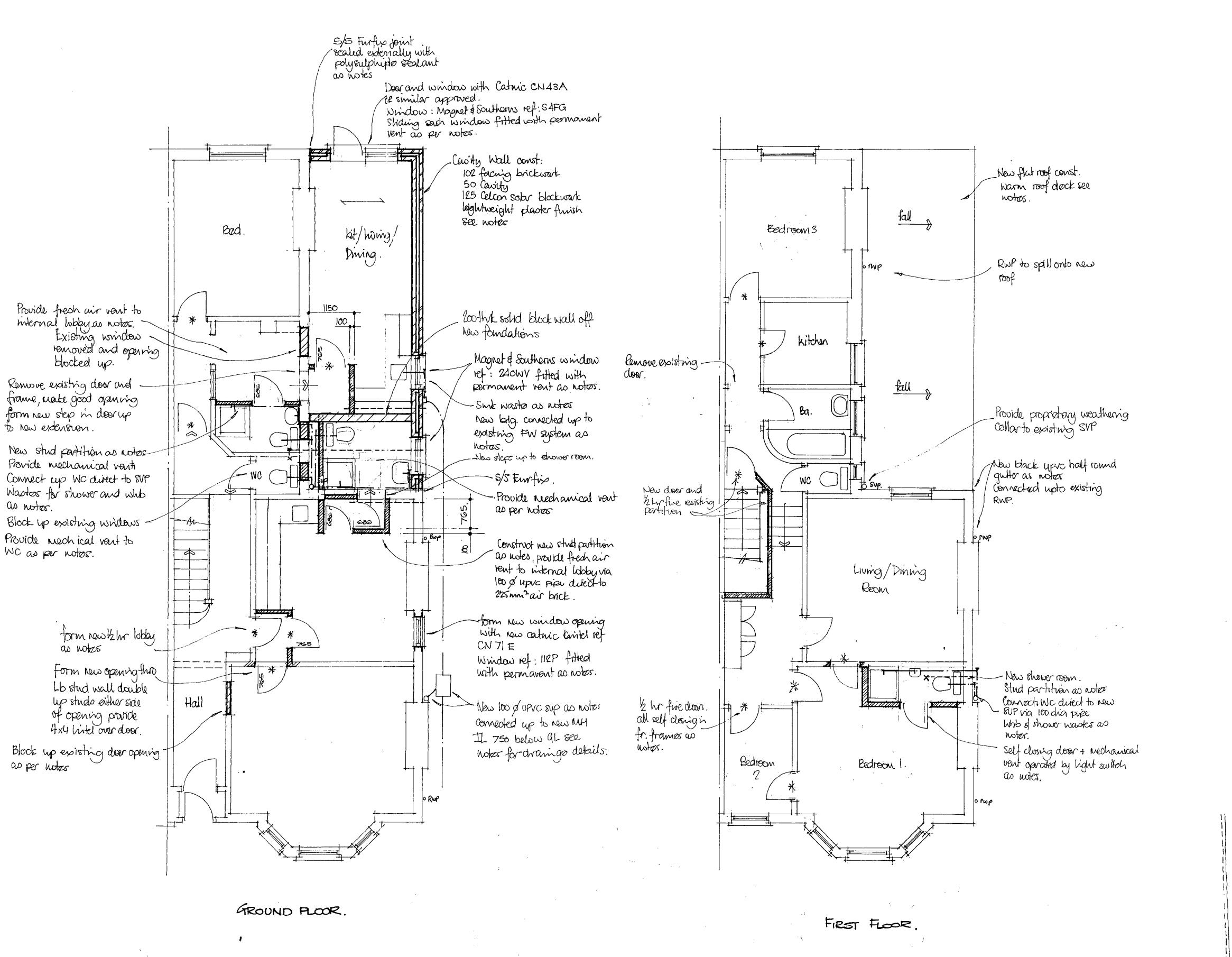
TIMBER PARTITIONS Studs to be 75mm x 50mm @ 400mm crs. with 75mm x 50mm head & sole plates.(2.4m high max.)
