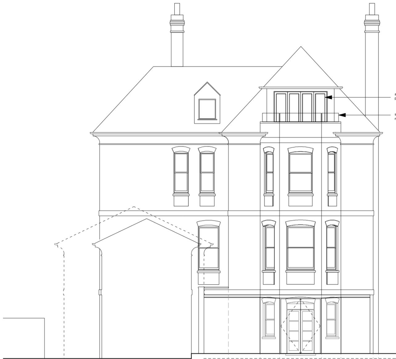
aluminium sliding doors to be replaced with painted timber glazed bi-fold doors
