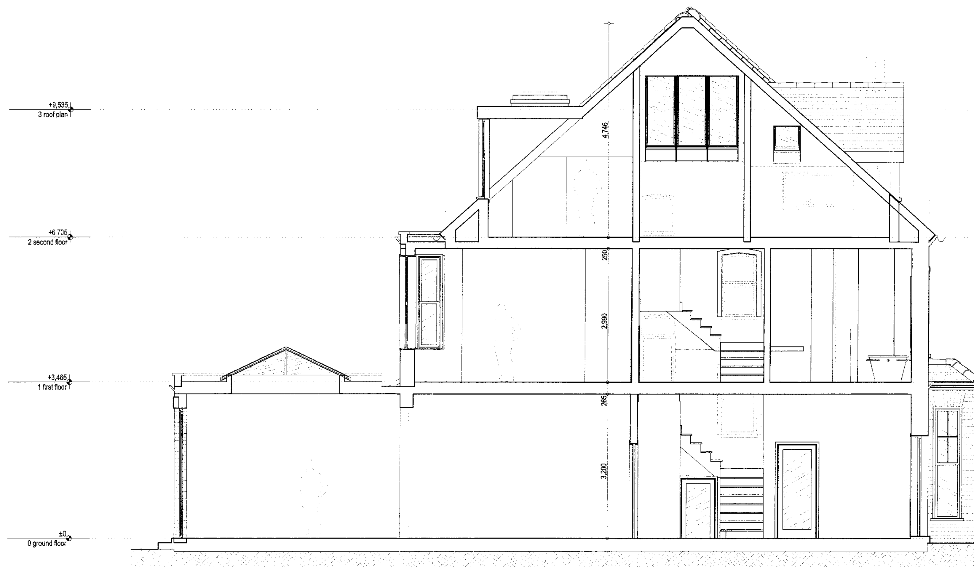
A longitudinal section as proposed 1:50
