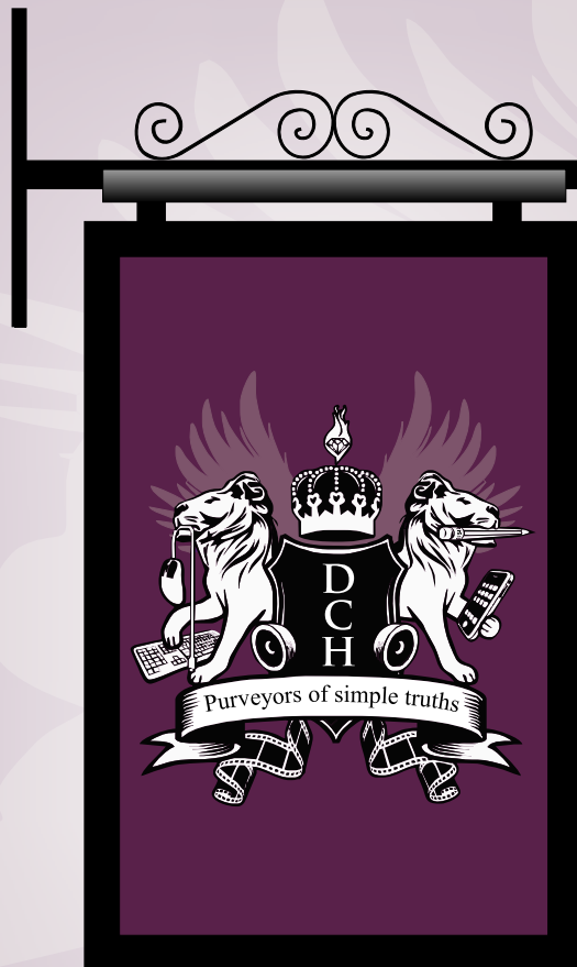
Sign 1 - Wall mounted projection sign with black simple scroll details, 600x900mm panel with black moulding and printed colour image. Externally illuminated by black trough lights.
