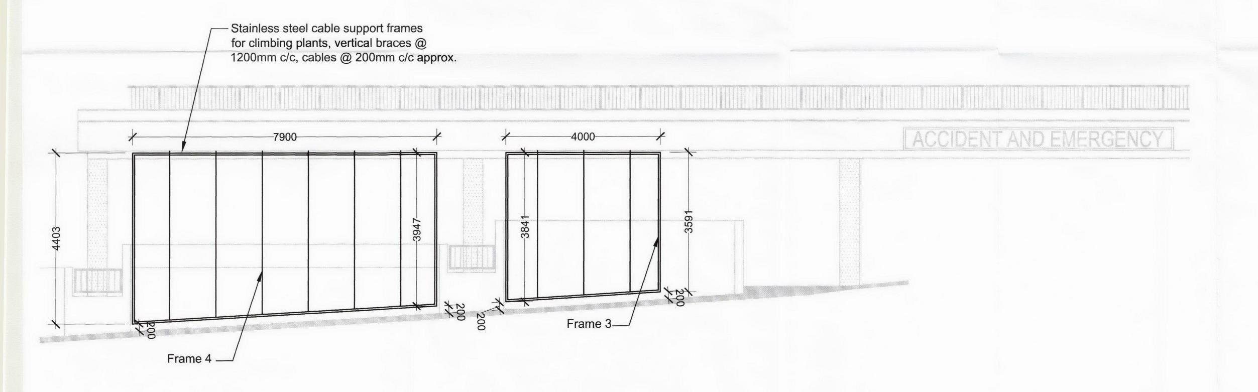
All frames fixed to face of brickwork at low level & u/s of concrete soffit at high level.
