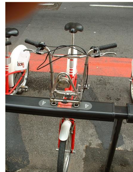
Figure 2.9: Bicing Docking Station
