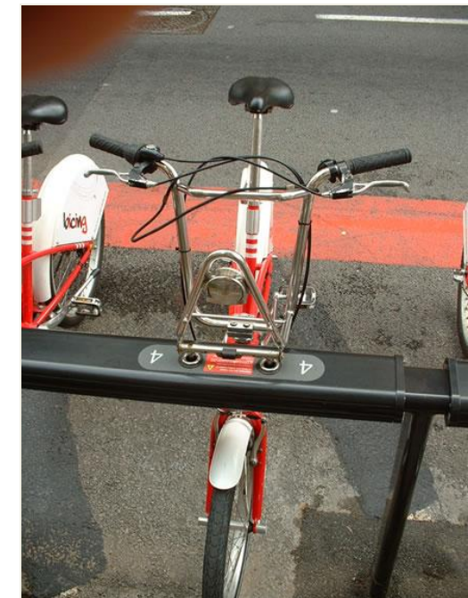
Figure 2.9: Bicing Docking Station
