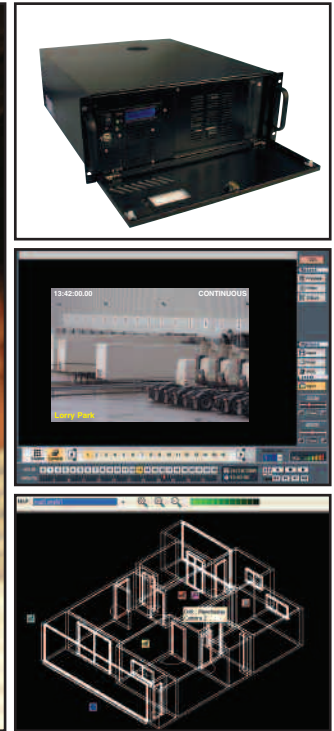
DVR 3000 series, remote menu navigation and a typical site map
