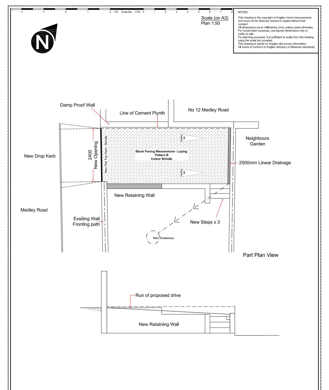
Ground levels will remain within 300mm of existing as necessary to create driveway.
