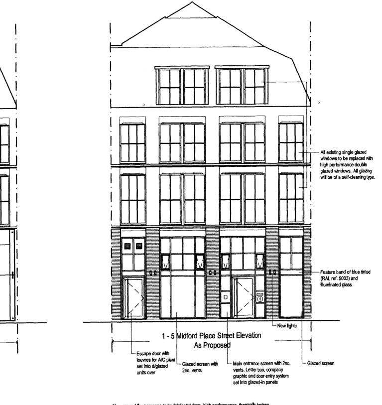
New ground floor screens to be fabricated from high performance, thermally broken, double glazed curtain walling (colour dark grey / bronze) complete with doors with full height pole handles. Glass clear except for slim feature band. All glazing wil be of a setf-cleaning type. Areas of screen will be fire rated in accordance with Building Regulation requirements
