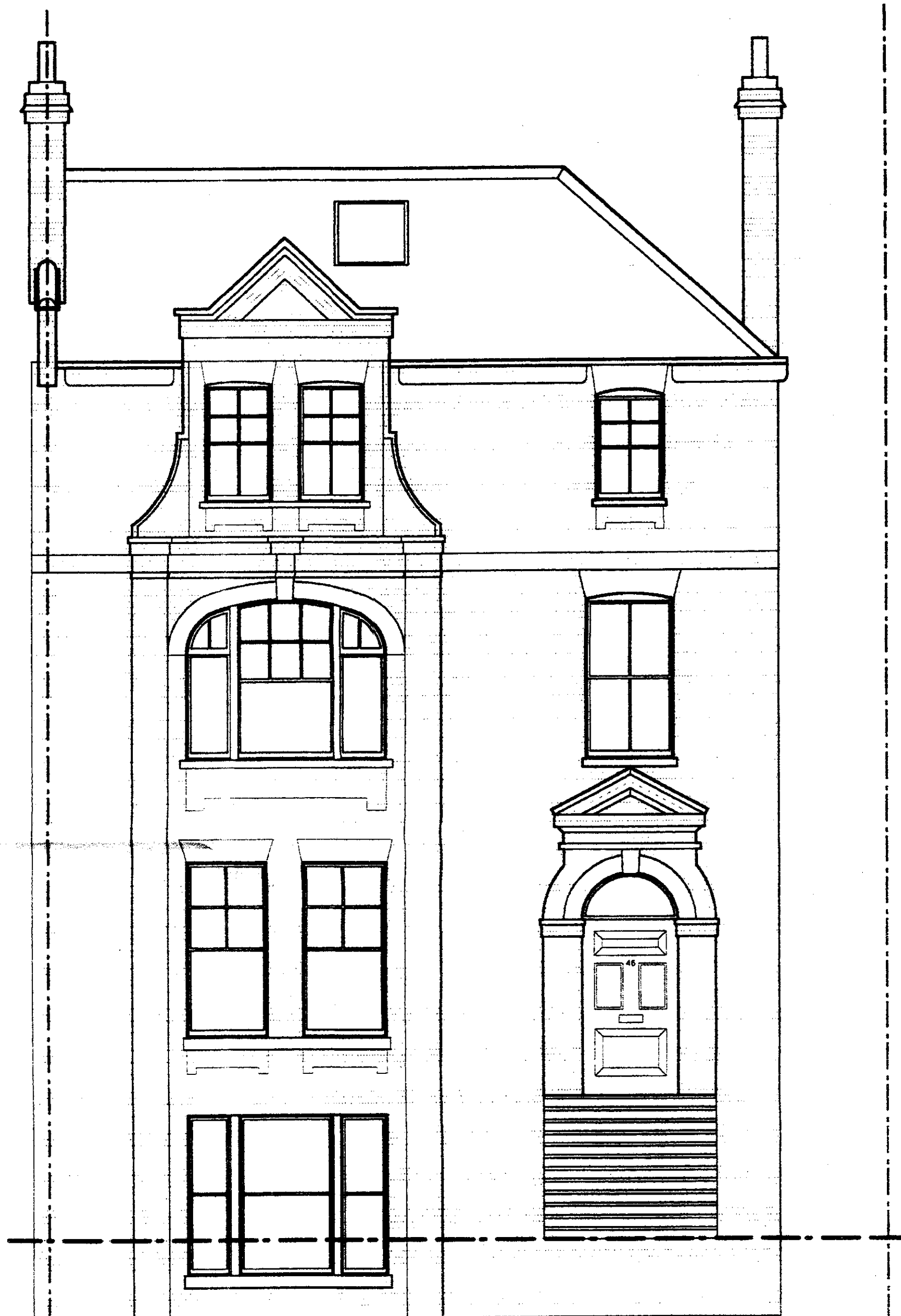
Existing West Elevation
