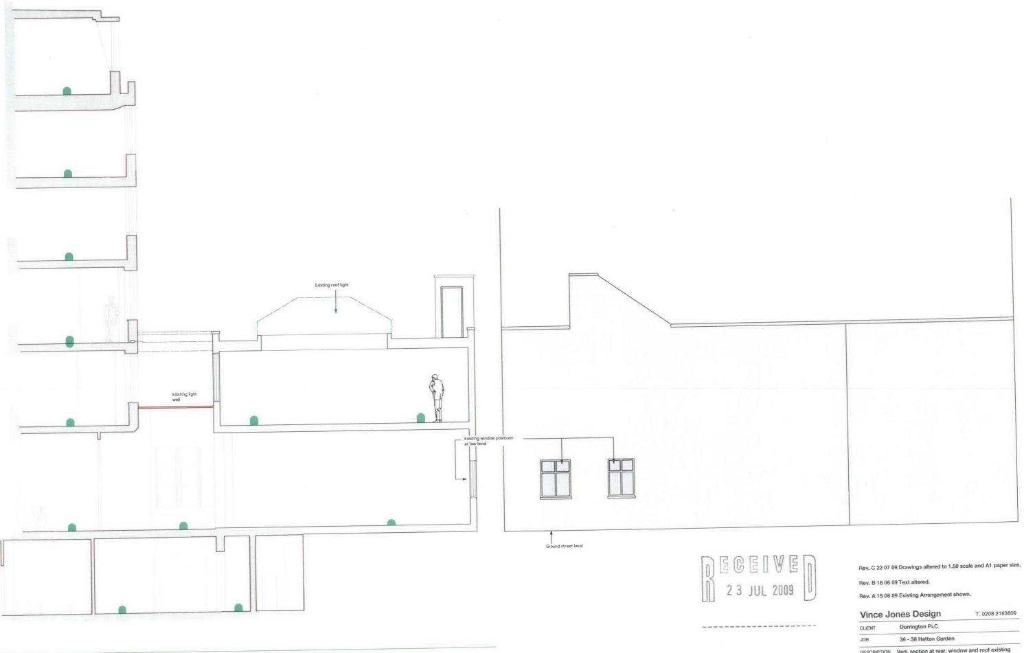
Existing Vertical section at AA 1.100 scale Showing Existing skylight at1st floor. Existing windows at ground floor. Existing Rear Elevation showing Existing window positions 1.100 scale
