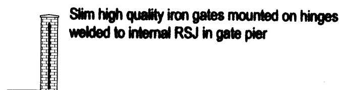
TYPICAL SECTION THROUGH GATE (SHOWING RELATIONSHIP TO PIER BEHIND) 1:50 scale
