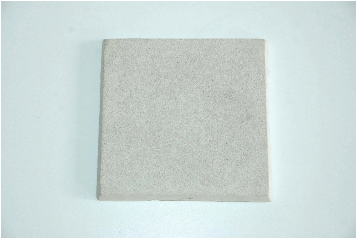
1 Swatch of GRC (Glass Reinforced Concrete) Indicative of surface texture - sand blasted and aggregate colour
