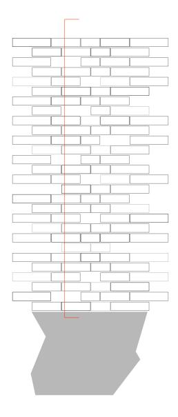
Notes 1. Height to match adjacent existing 2. Perforated brickwork to allow sun to penertrate.
