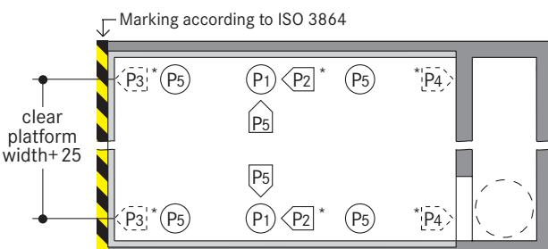
\* The force P2 is only given when the pillars are fitted to the side walls.
