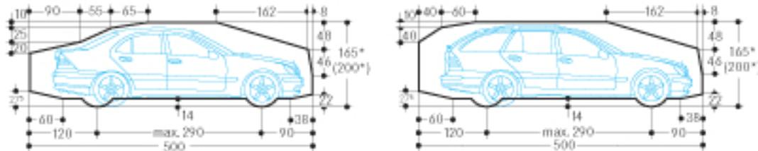
\* The total car height includes roof rail and antenna fixture and must not exceed the mentioned max. height dimension.
