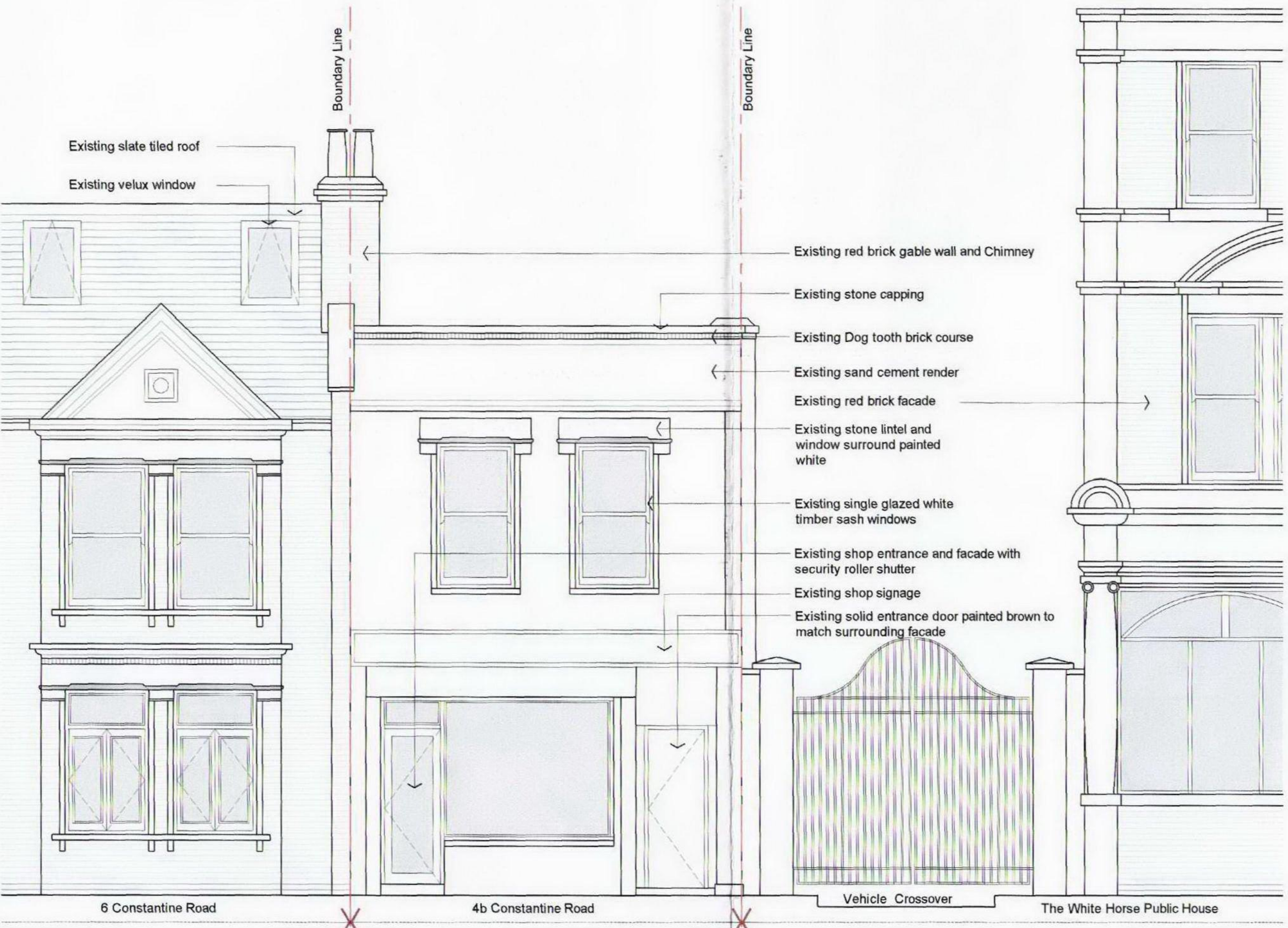
Existing Front Elevation Scale 1:50 @ A1
