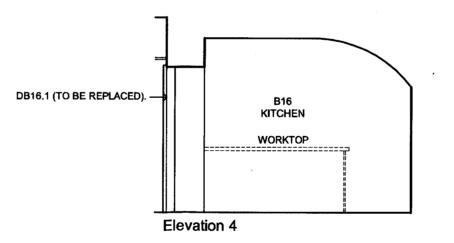
ITEMS TO BE STRIPPED OUT AND REMOVED GENERALLY SHOWN LIGHT GREY LINE AND / OR DOTTED. SEE ALSO DEMOLITIONS PLAN AL(21)D01.
