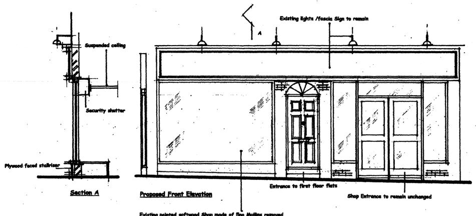
Existing painted softwood Shop made of Sno Mullins removed And replace with new side, header and window board With one single sheet of 12.8mm clear glass
