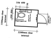
Floor plan detail of disabled W.C to part M regulations. Disabled W.C to have emergency pull cord system, with audible and visual signal.
