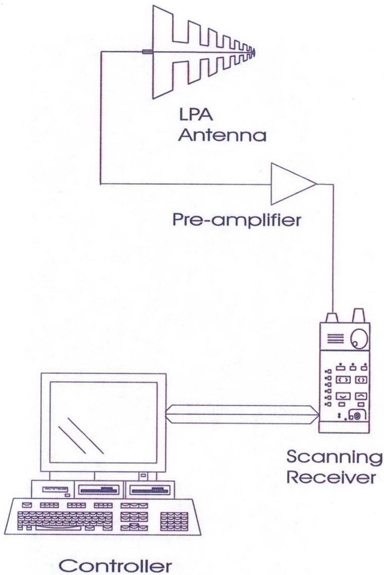
Fig.A.2 : Test Schematic - Signal Strength (450MHz - 650MHz)
