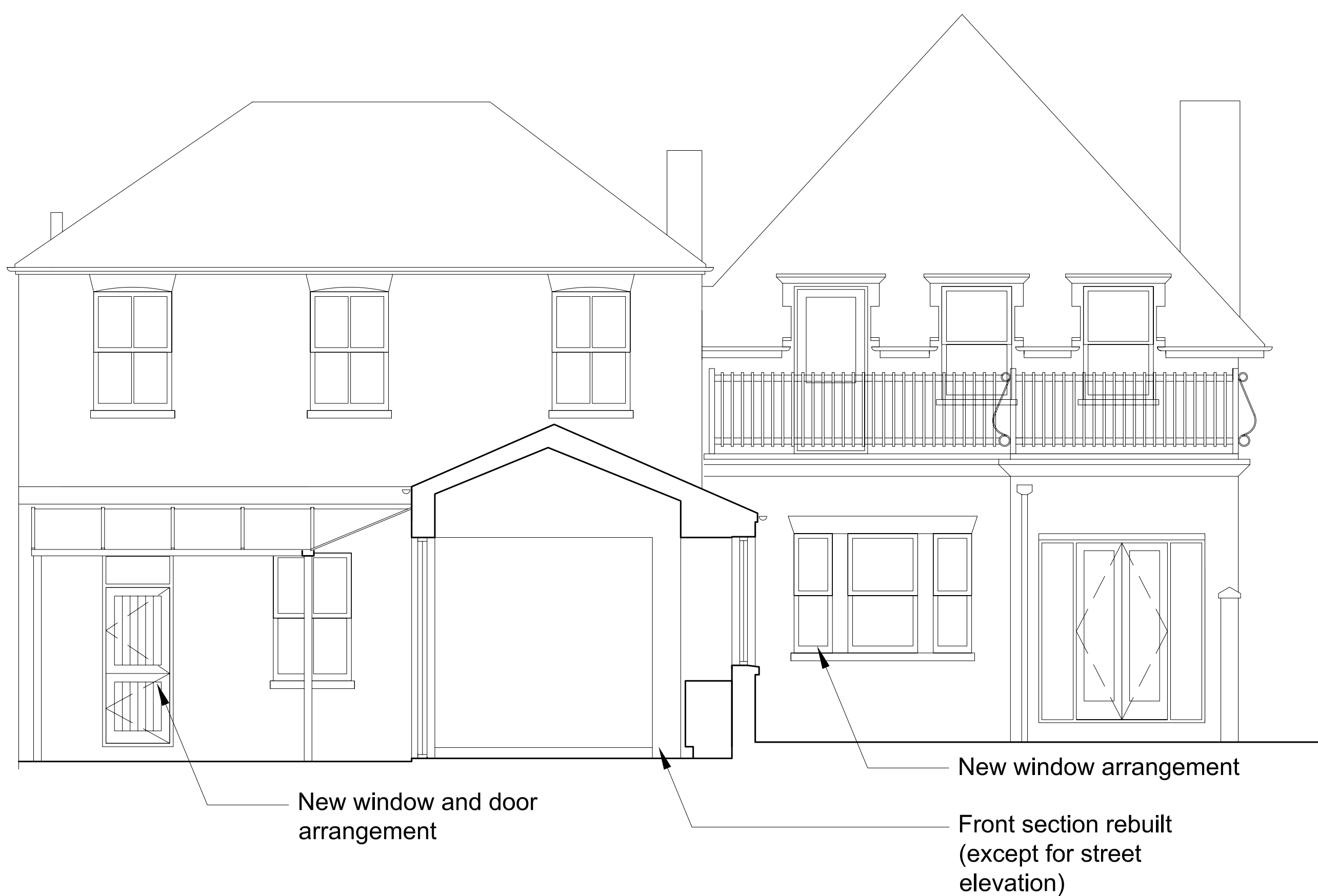
Courtyard (East) Elevation / Section C:C
