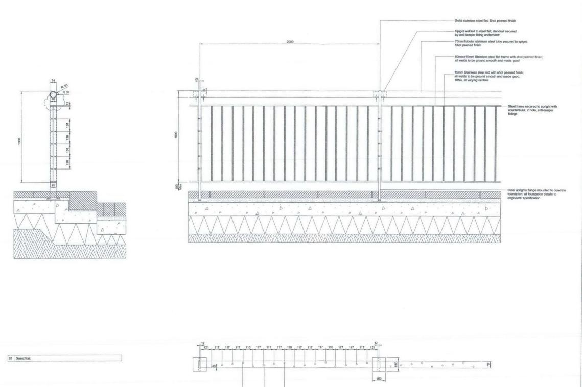
15mm Stainless steel rods with shot peened finish; —all welds to be ground smooth and made good.
