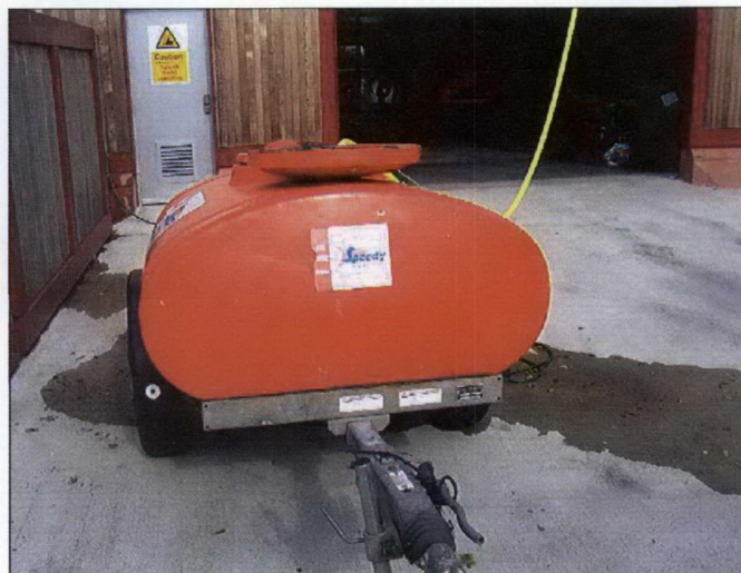
In situations where the mains water pressure is found to be insufficient, a Bowser can be used together with a pump, to provide the required pressure to roof level.
