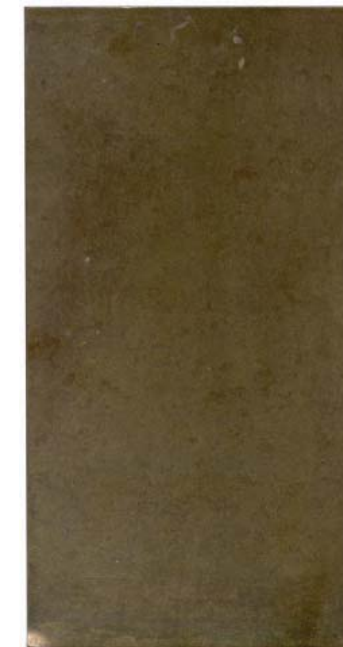
Sample of brass when weathered. After a period of 3 months the brass will have acquired the patination as shown above. Individual shingles will weather with slight variations in colour, giving a texture that will reflect the condition found in the concrete blocks that form the plinth to Levita House.
