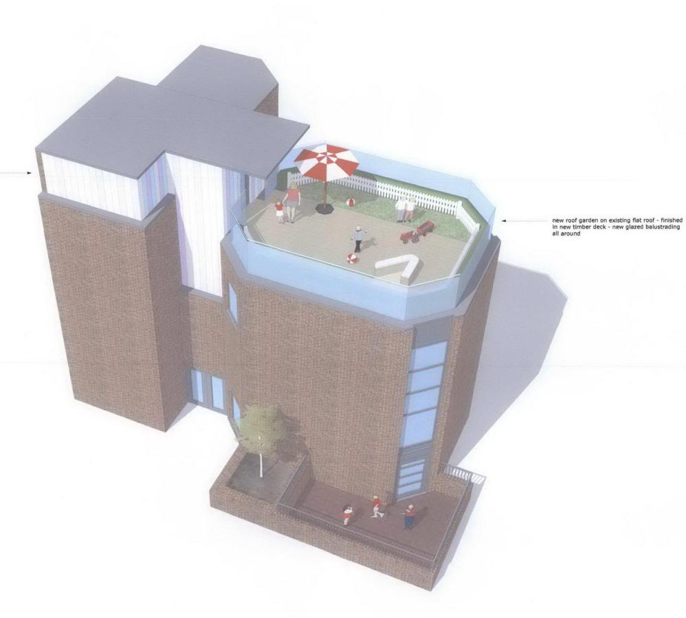
new rooftop extension providing access to roof garden - side elevations clad in — glazing system
