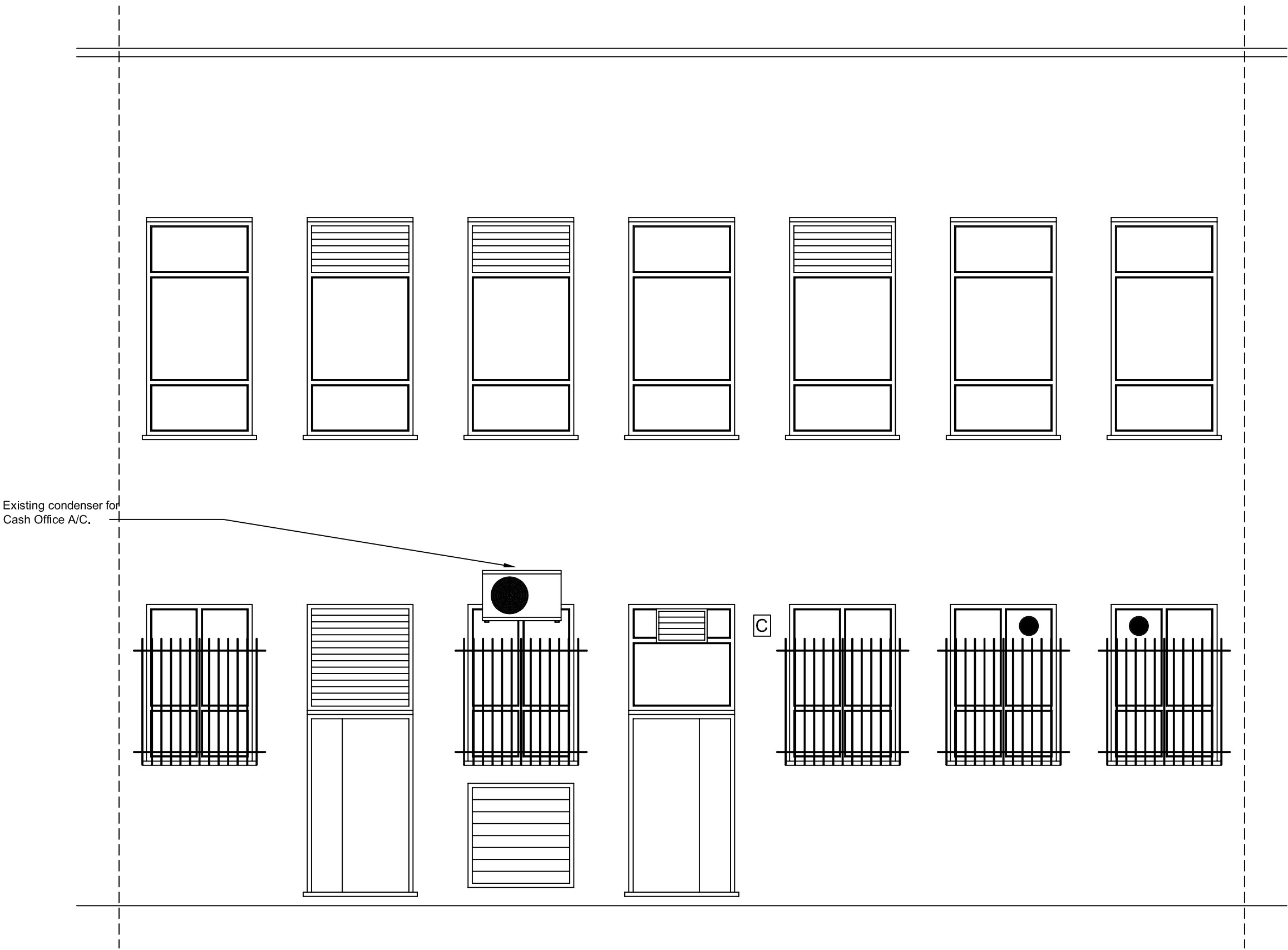
Existing Rear Elevation
